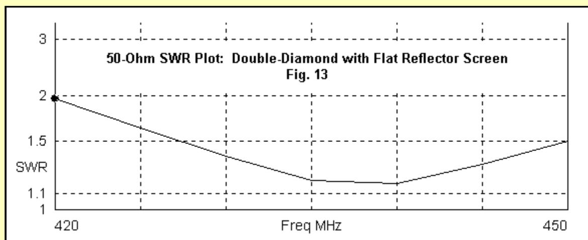
The resulting SWR curve in **Fig. 13** shows excellent coverage of the band, especially the upper end. By judiciously altering the dimensions of the single double-diamond, one can adjust the resonant position and hence the shape of the SWR curve to favor any part of the band.
