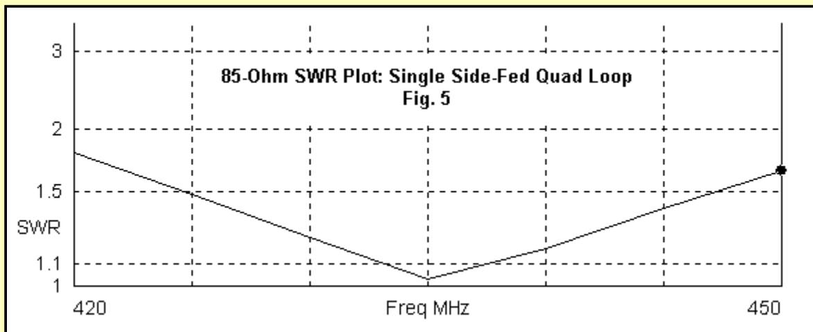
**Fig. 5** shows that the single diamond loop is--using a 4-mm diameter--a potentially wide-band antenna. The SWR curve is partly a function of the large element diameter when measured as a fraction of a wavelength.
