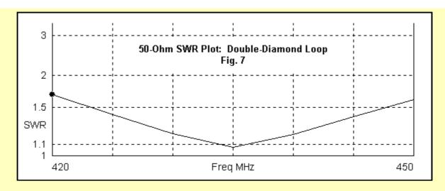
Over the entire 420-450-MHz band, the performance of the double-diamond remains quite stable, with only about a 0.2 dB change in maximum free-space gain from one end of the band to the other. The following table also shows that the half-power beamwidth is also quite stable, varying only about 2-3 degrees across the band.
