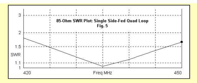
**Fig. 5** shows that the single diamond loop is--using a 4-mm diameter--a potentially wide-band antenna. The SWR curve is partly a function of the large element diameter when measured as a fraction of a wavelength.
