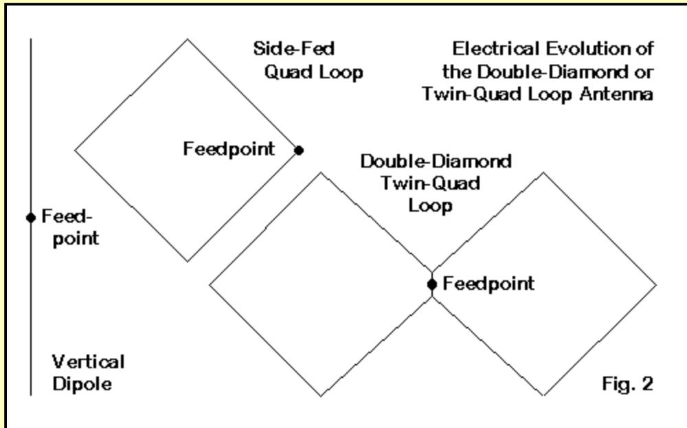
The beginning of the double-diamond quad loop abides in the simple vertical dipole. A 4-mm diameter aluminum vertical dipole for 432 MHz in free space will show a gain of about 2.1 dBi and a resonant feedpoint impedance of about 72.5 Ohms. These values are the touchstone for all further work, and the circular H-plane pattern of **Fig. 3** serves only as a reminder.
