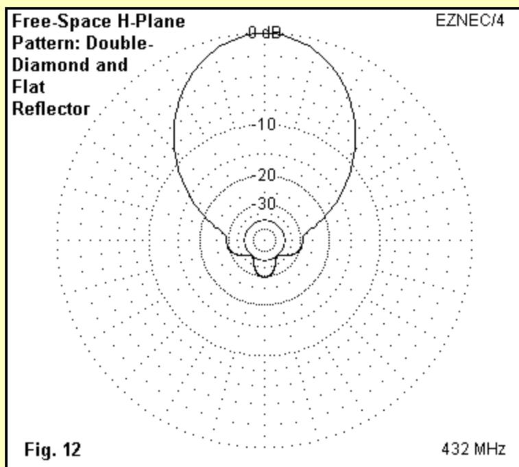
The following table of modeled values shows the flatness of performance of the array when used with the smallest of the screen sizes.
