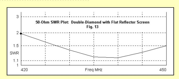
The resulting SWR curve in **Fig. 13** shows excellent coverage of the band, especially the upper end. By judiciously altering the dimensions of the single double-diamond, one can adjust the resonant position and hence the shape of the SWR curve to favor any part of the band.
