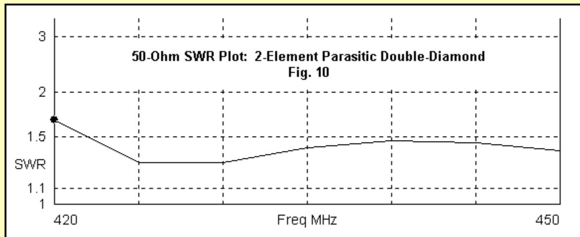
**Fig. 10** provides the 50-Ohm SWR curve for the array. SWR reaches about 1.7:1 at the low end of the band, but from 425 MHz upward, it levels off in the 1.28:1 to 1.50:1 range. Like most quad beams, the SWR operating curve is much flatter than the performance (gain and front-to-back ratio) curves.
