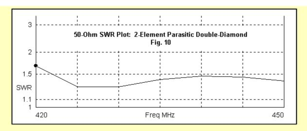
**Fig. 10** provides the 50-Ohm SWR curve for the array. SWR reaches about 1.7:1 at the low end of the band, but from 425 MHz upward, it levels off in the 1.28:1 to 1.50:1 range. Like most quad beams, the SWR operating curve is much flatter than the performance (gain and front-to-back ratio) curves.
