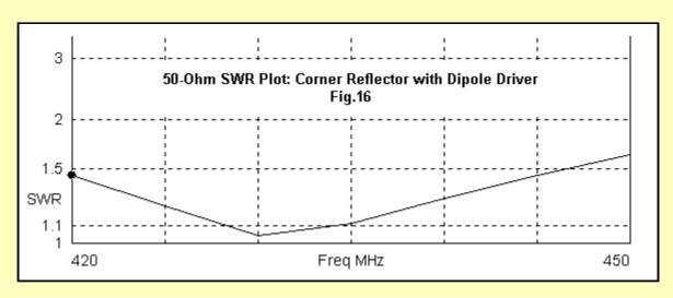
Equally, like the double-diamond array, the performance characteristics promise to be very consistent across the entire 420-450-MHz spectrum. The follow tables provides samples.
