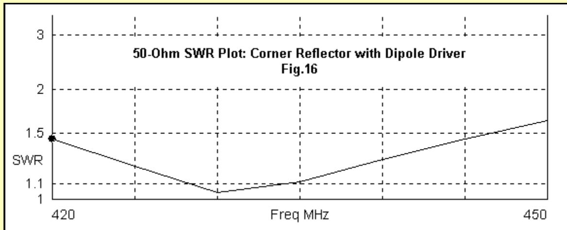
Equally, like the double-diamond array, the performance characteristics promise to be very consistent across the entire 420-450-MHz spectrum. The follow tables provides samples.
