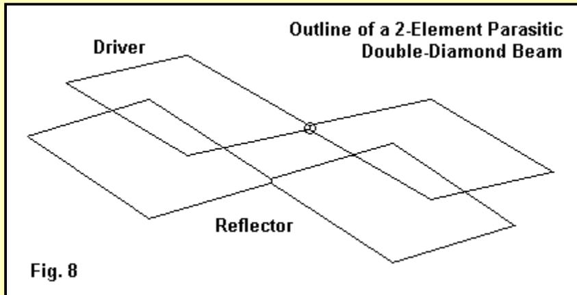
From the 1/4" material, I modeled a 2-element parasitic array consisting of a driver and a reflector, as outlined in **Fig. 8**. Like standard quads, the reflector of a double-diamond quad must be further to the rear of a driven element than for a Yagi with linear elements. The final spacing was about 0.22 wavelength.
