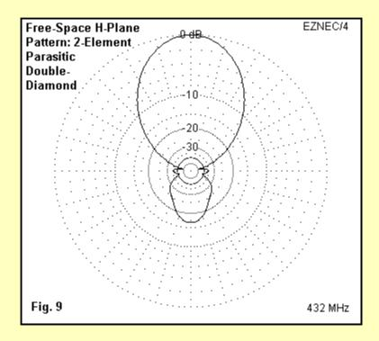
The following table of values taken across the full 420-450 MHz band shows that the performance peaks at mid-band and falls off toward the band edges. Maximum gain occurs about 5 MHz below the maximum front-to-back frequency, a common phenomenon with any 2-element quad array. The performance curve is not unlike that of a 4-element Yagi designed to cover the entire 420-450 MHz band.
